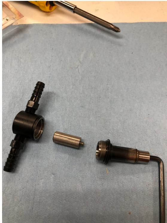
Separate the parts and remove any debris present.
