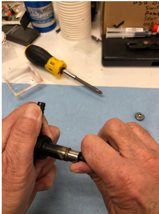
Unscrew the stem from the valve body
